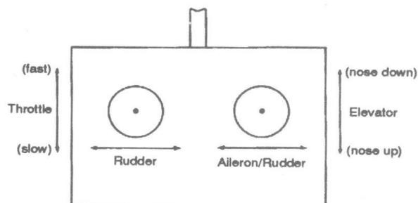
Alongside each of these controls on the transmitter are sliding levers which are the trims for each control. What they effectively do is to alter the neutral position of the related control so that by using them when the aircraft is in the air you can cancel out any out-of- balance forces which make the aircraft tend to climb/dive or turn.
