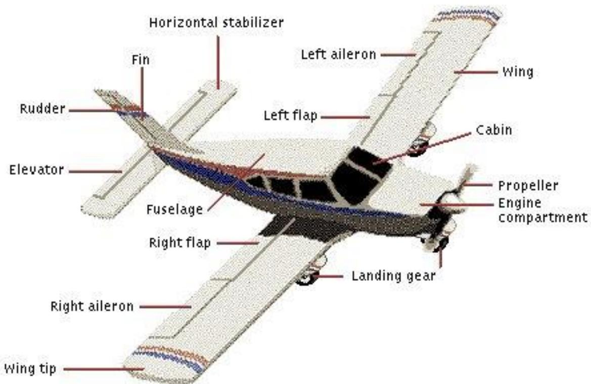
Sometimes we will hear the term "airframe" being used. Simply the airframe is the complete structure of an aircraft, less the engine, instruments and ancillary equipment such as radios. So let's take a look at each of these parts.
